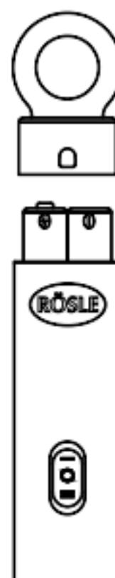
Put the ring back onto the handle and lock it in place so that the ring aperture aligns with the RÖSLE logo.
